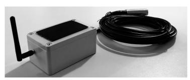
AGWAN LoRaWAN network. Once received by the base-station/gateway at the farmer's residence, this is uploaded over the internet to the AGWAN Cloud and converted into a depth that the farmer can view on the AGWAN App. Users can set alarm limits so that text message notifications can be received should water levels go beyond maximum or minimum thresholds.
